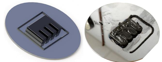
Digital model of sample part (left) and printed part (right)
